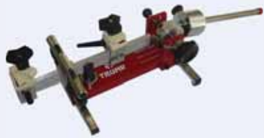
SM-B1 Table-top, 4-point drop-weight tension system, flying clamps
